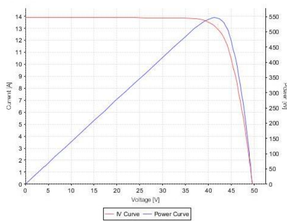
Fig. 5 IV curve of module No.1 Serial number: AS22200108899
